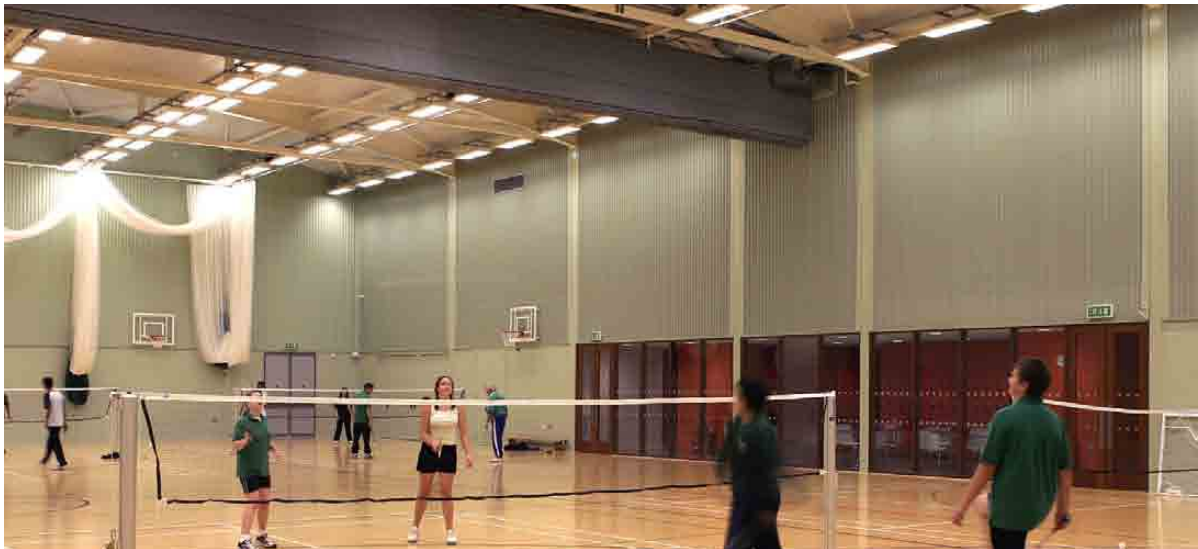
Acoustic dividing screen at the centre point of a 6-court hall on a school site allows the space to be divided into two teaching spaces
